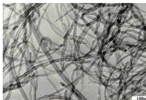
Fig. 1: TEM image of multi-walled carbon nanotubes that functionalized with carboxyl groups.
