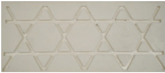
Fig. 2: Silicone mold used for fabrication of grid composite structures.
