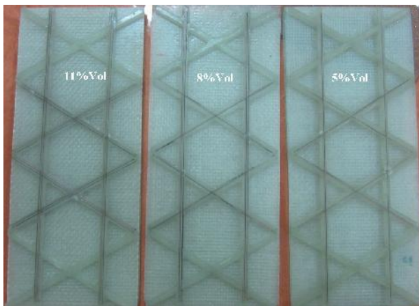
Fig. 3: Self-healing specimens containing 5, 8 and 11 volume percent of self-healing materials.
