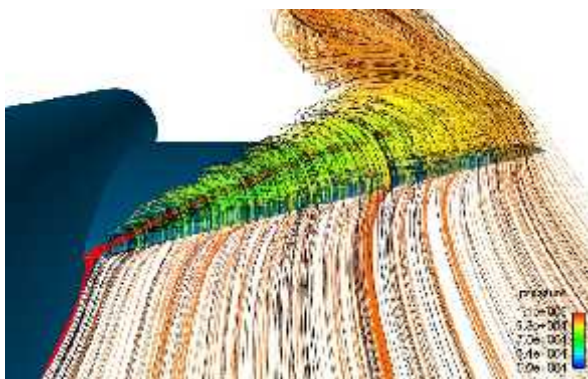
Figure. 3: Perspective view of vortex structure, some streamlines are colored in black for better display.
