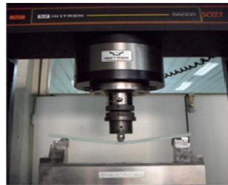
Fig. 3: Single-point bending test with INSTRON 5500R
