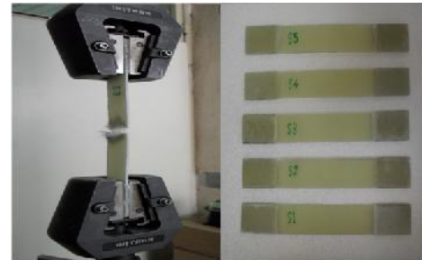
Fig. 4: Tensile test samples and tensile test of sample 3#
