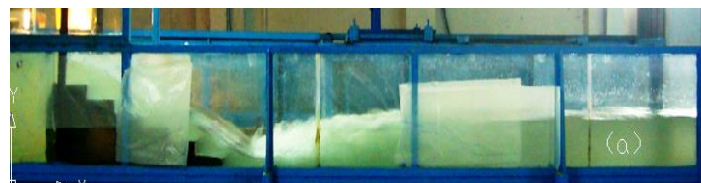
Figure 3. Flow over the spillway and the downstream hydraulic jump of experimental model.
