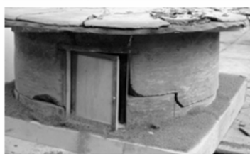
3-4 to 3-8 Earthquake tests with models of square and circular shape (Minke 2001)
