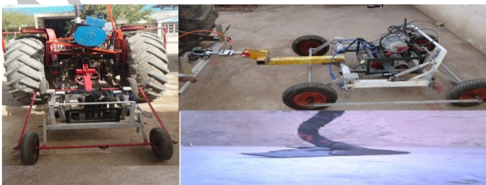
Fig.1. The experimental tillage (right) - tillage blade and stem (left)
