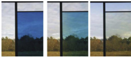
Fig. 2 The color change of electrochromic and thermochromic windows
